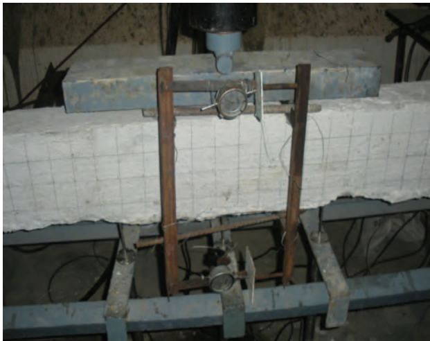
Fig 5. Dial gauge arrangement to compute strain of beam
