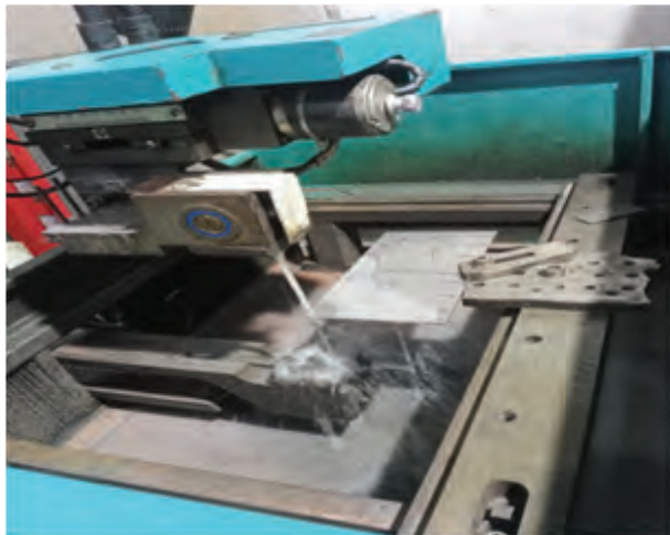
Fig.4: Fixing of workpiece on machine table
