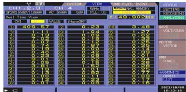
Figure 4: VFD input voltage harmonic measurement at full load
