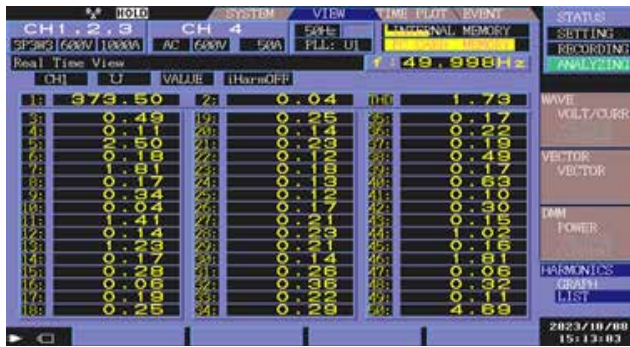
Figure 7: VFD output current harmonic measurement at full load
