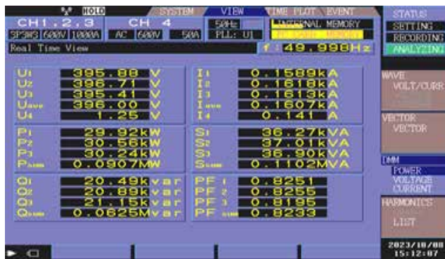
Figure 8: Output parameters of VVVF fed induction motor drives dynamic performance at full load
