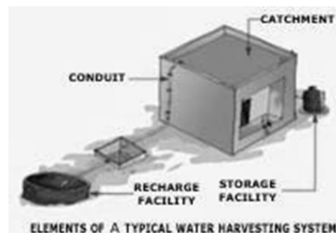
Fig.1 Rain Water Harvesting System
