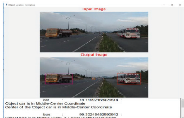
Fig. 4. YOLOv8 based object detected and OLEA based object located Road image
