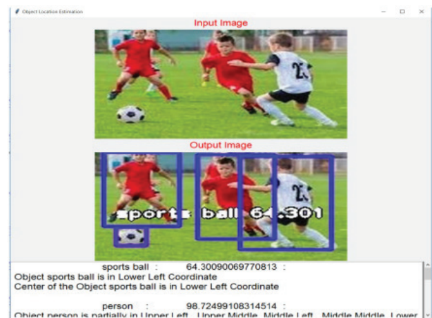
Fig. 2. YOLOv8 based object detected and OLEA based object located play ground image
