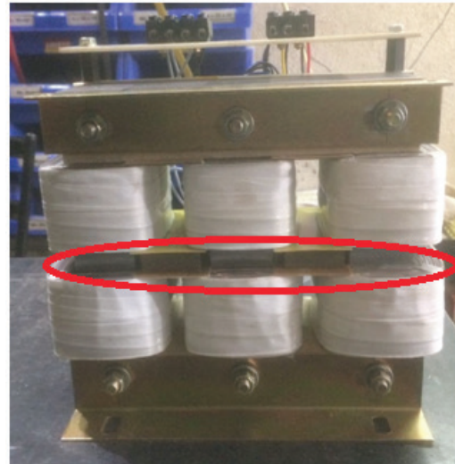
Fig. 2 Special design of core and windings in transformer
