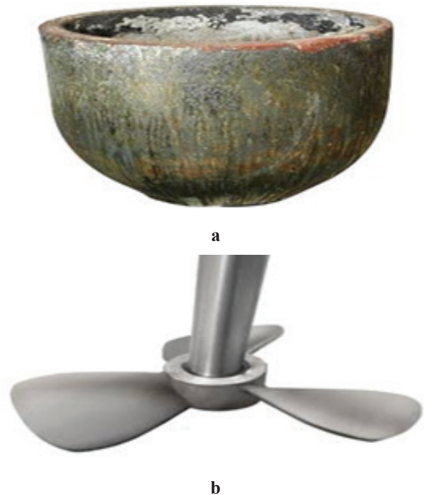
Fig 10. (a) Ceramic Crucible; (b) Stirrer with Three Blade Impeller
